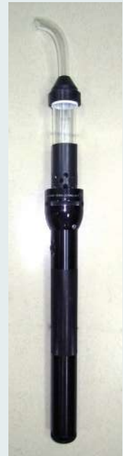
Figure 3.2: Battery operated aspirator
